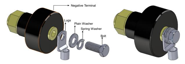
Figure 1.Connecting washers, lugs and bolts to negative terminal of Module
